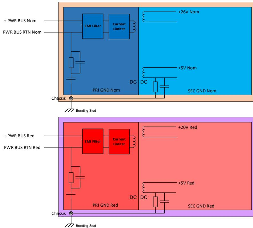
The Power Supply Unit has a primary ground and one single secondary ground for all type circuitries (analogue and digital). Between primary and secondary ground there is a galvanic isolation. The primary ground is routed through the EMI: this is the star-point and is connected to the bonding stud. Secondary ground is connected by 5.6M//10nF to chassis.
